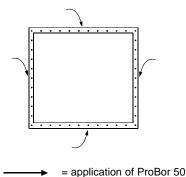
Figure 16: ProBor 50 applied to masonry
